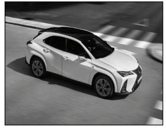
variable transmission (CVT) is hooked up to standard all-wheel drive (AWD) via a rear electric motor. Note the 300h is not a plug-in hybrid and generates it own hybrid power on board, The 2025 Lexus UX 300h
